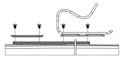
**STEP 4.** Tighten frame screws to manufacturers recommended torque (See notes). Check clearances with bottle cage and accessories installed before riding.
