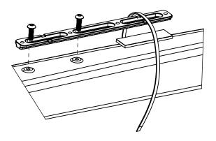
**STEP 3.** Mount accessories and bottle cages to the 3-slot base using "short" screws. Use low profile zip tie and zip tie channels for additional stability at unsupported end of base.
