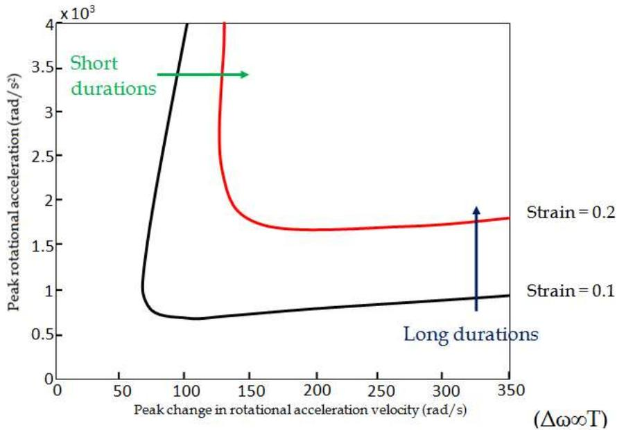
Figure 2-3: Acceleration vs. time injury tolerance curve [2]
