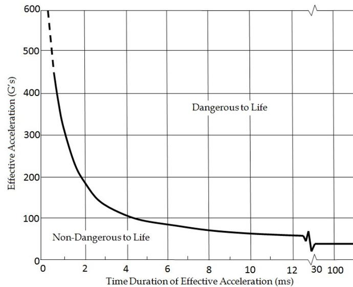
**Figure 2-1: Wayne State Tolerance Curve [1]**
