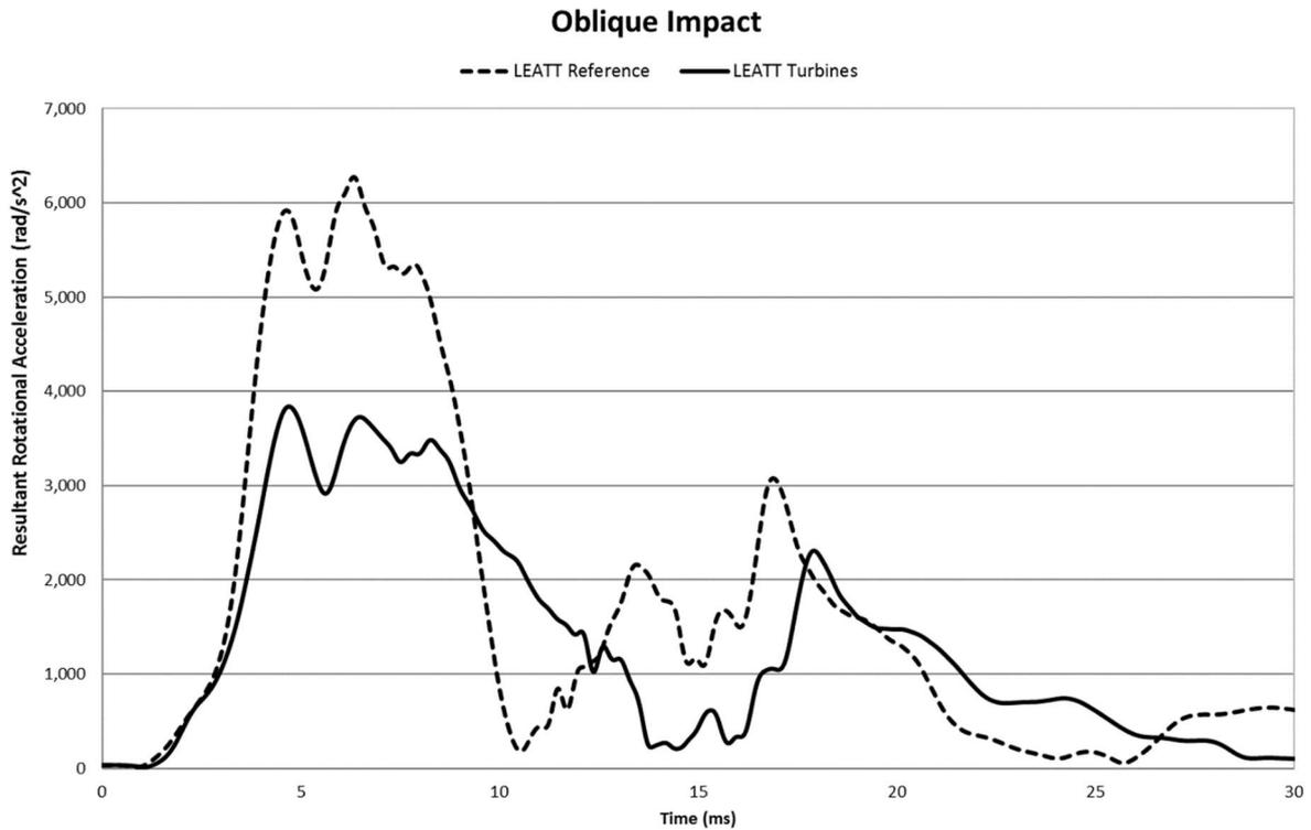
**Figure 4-3: 6.1 m/s rear oblique impact - illustration of transferred energy reduction**
