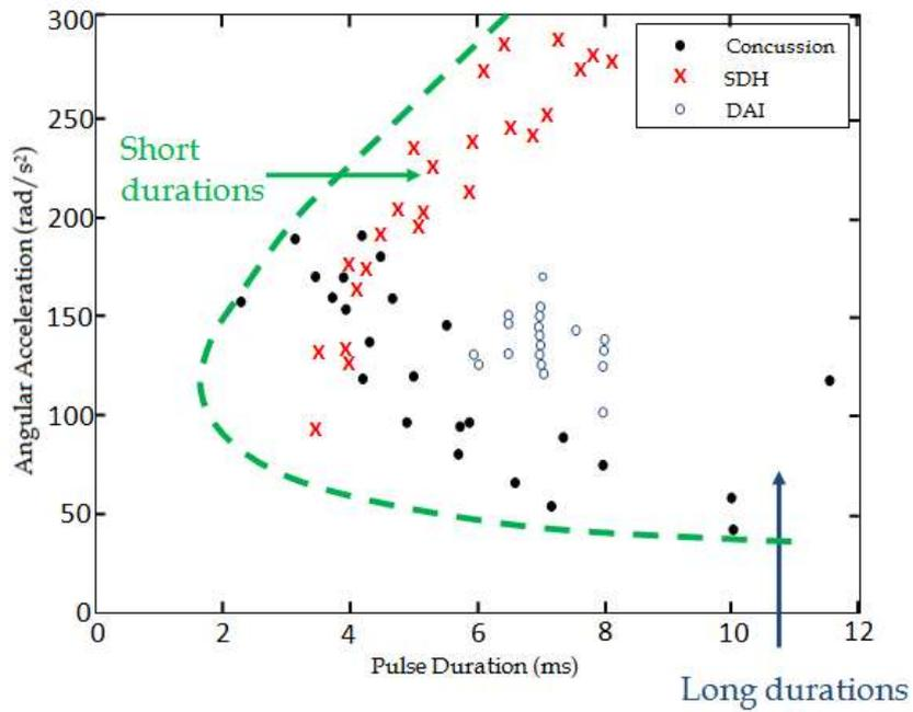
Figure 2-2: Acceleration vs. time injury tolerance curve [2]
