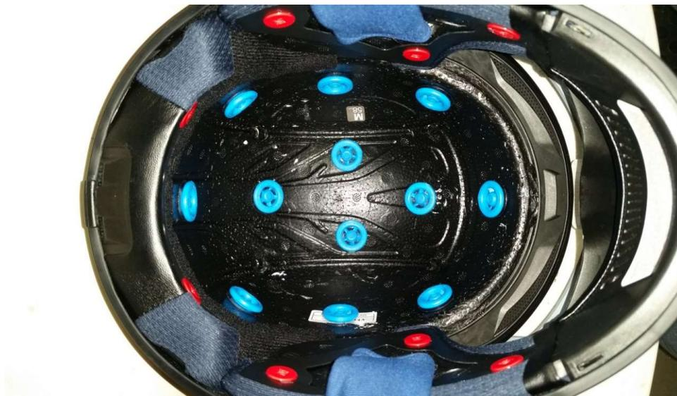
**Figure 3-3: Turbines in place within the EPS structure**
