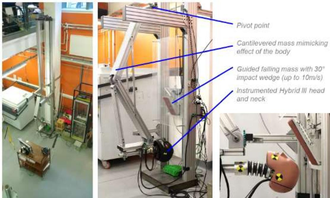
**Figure 4-1: Oblique impact helmet test rig**
