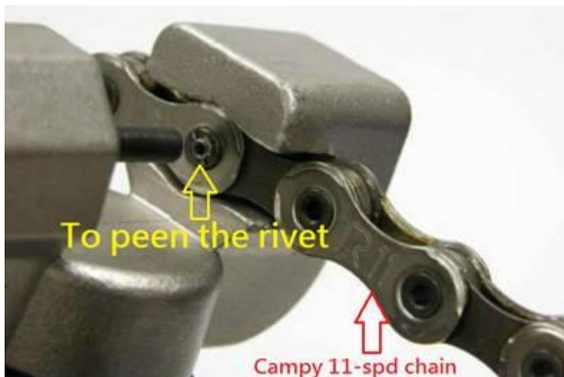
Therefore, the chain tools (All speeds chain tool, LINK11, Tool Monster) that we say : for 11-spd means equipped "rivet anvil" for user to do the "peening" work for Campy's chain.
