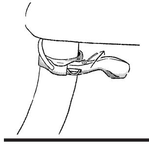
PULL THE CABLE THROUGH THE LEVER AND HOLE IN THE BARREL NUT UNTIL THE CABLE IS TIGHT.
