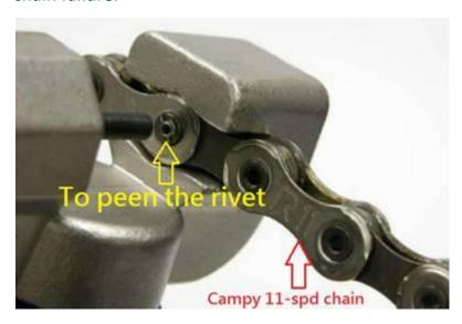
Therefore, the chain tools (All speeds chain tool, LINK11, Tool Monster) that we say: for 11-spd means equipped "rivet anvil" for user to do the "peening" work for Campy's chain.
