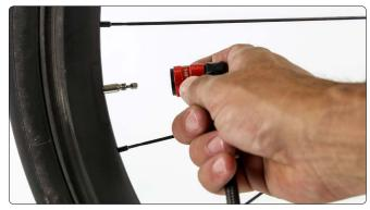
Open Presta valve and pull sleeve back on ABS2 chuck.
