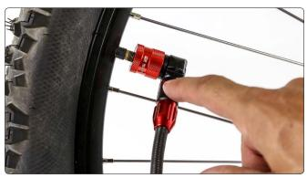
Inflate to desired pressure and use the bleed valve to adjust pressure.
