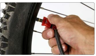
Slide sleeve forward and thread onto Shrader valve.
