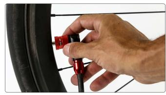
Press onto valve, slide sleeve forward and rotate sleeve 1/4 turn to seal.
